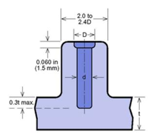
It is suggested avoiding bosses that merge into sidewalls because they can form thick sections that lead to sink. Proper bosses should be positioned away from the sidewall, and if needed, use connecting ribs for support. Try using open boss designs for bosses near a standing wall.
