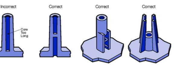
Options to reduce excessively-long core pins.
